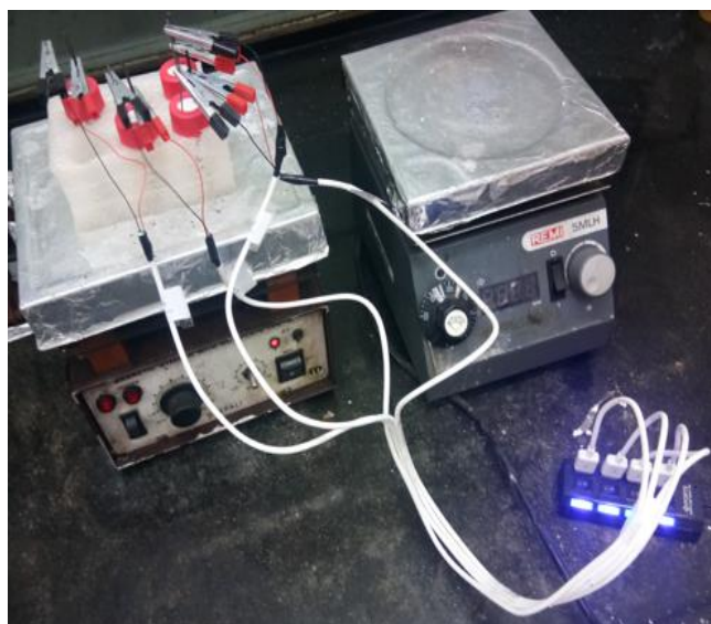
Figure 1. Multiple reaction assembly.
