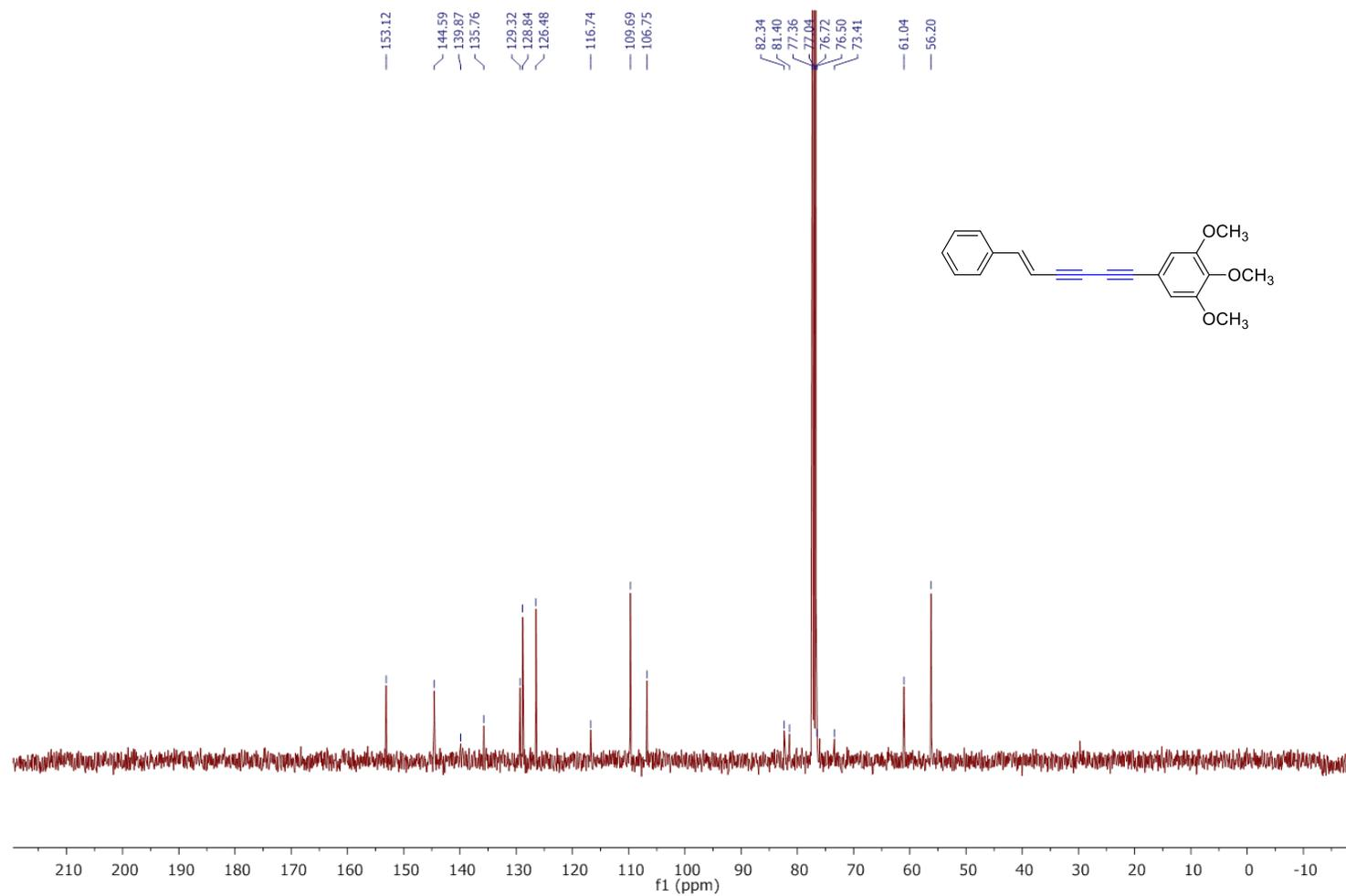
Fig. 38.  $^{13}\text{C}$ -NMR-spectrum of compound **2s** (101 MHz,  $\text{CDCl}_3$ , 298K)
