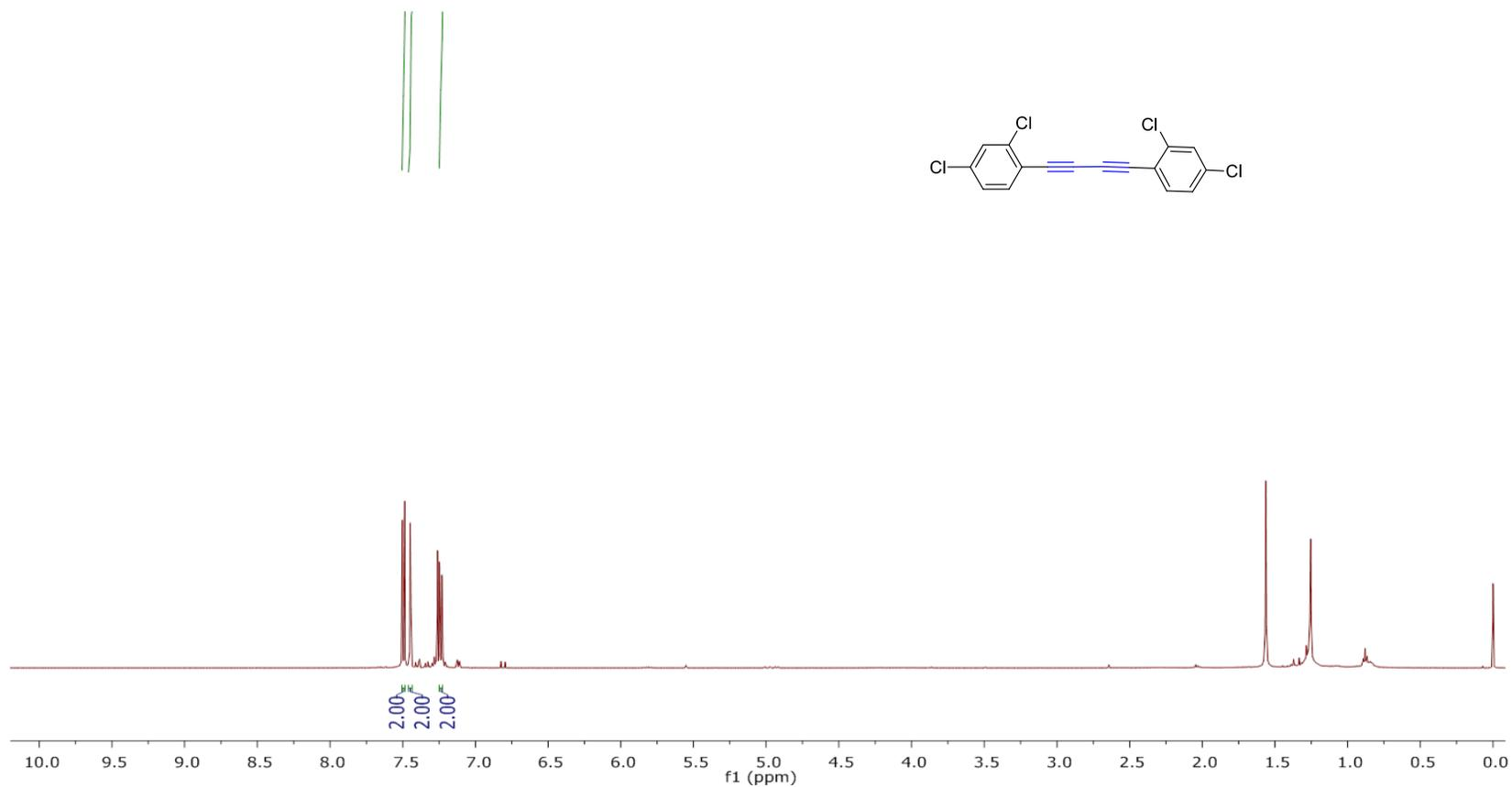
Fig. 25. <sup>1</sup>H-NMR-spectrum of compound **2m** (500 MHz, CDCl<sub>3</sub>, 298K)
