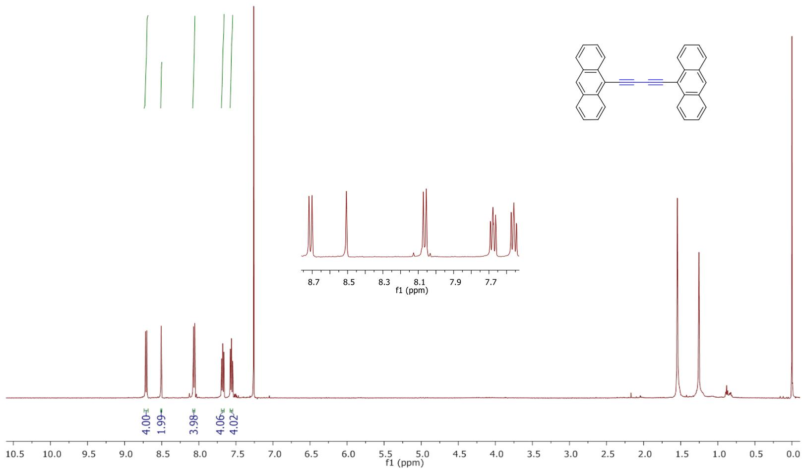
Fig. 15.  $^1\text{H-NMR}$ -spectrum of compound **2h** (500 MHz,  $\text{CDCl}_3$ , 298K)
