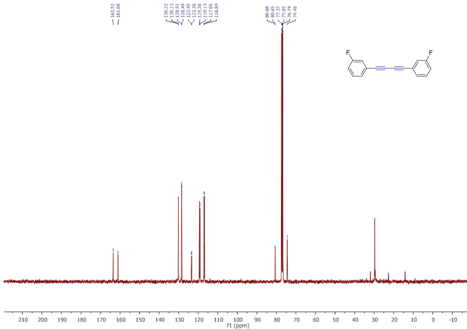
Fig. 20.  $^{13}\text{C}$ -NMR-spectrum of compound **2j** (101 MHz,  $\text{CDCl}_3$ , 298K)
