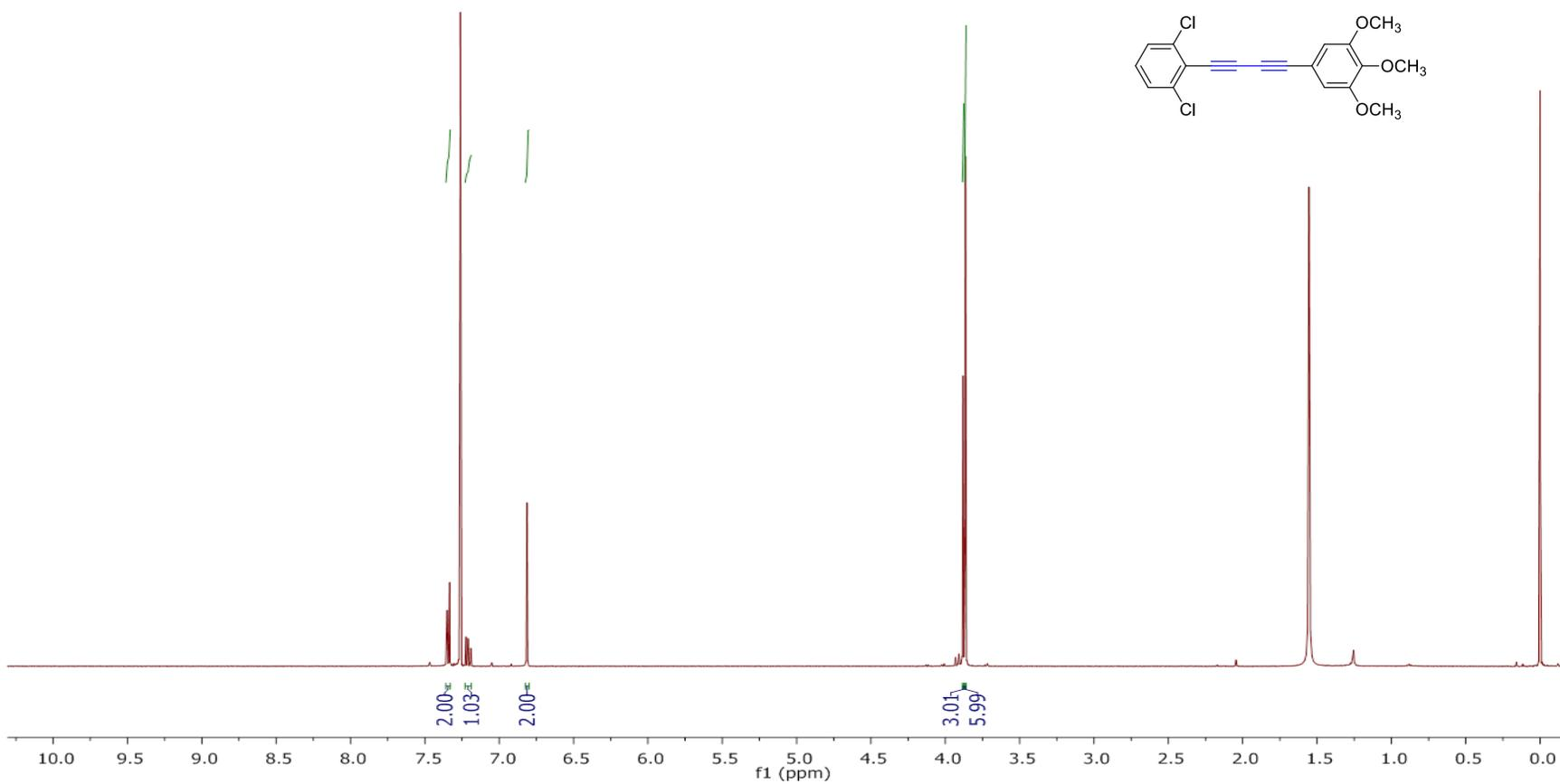
Fig. 35. <sup>1</sup>H-NMR-spectrum of compound **2r** (500 MHz, CDCl<sub>3</sub>, 298K)
