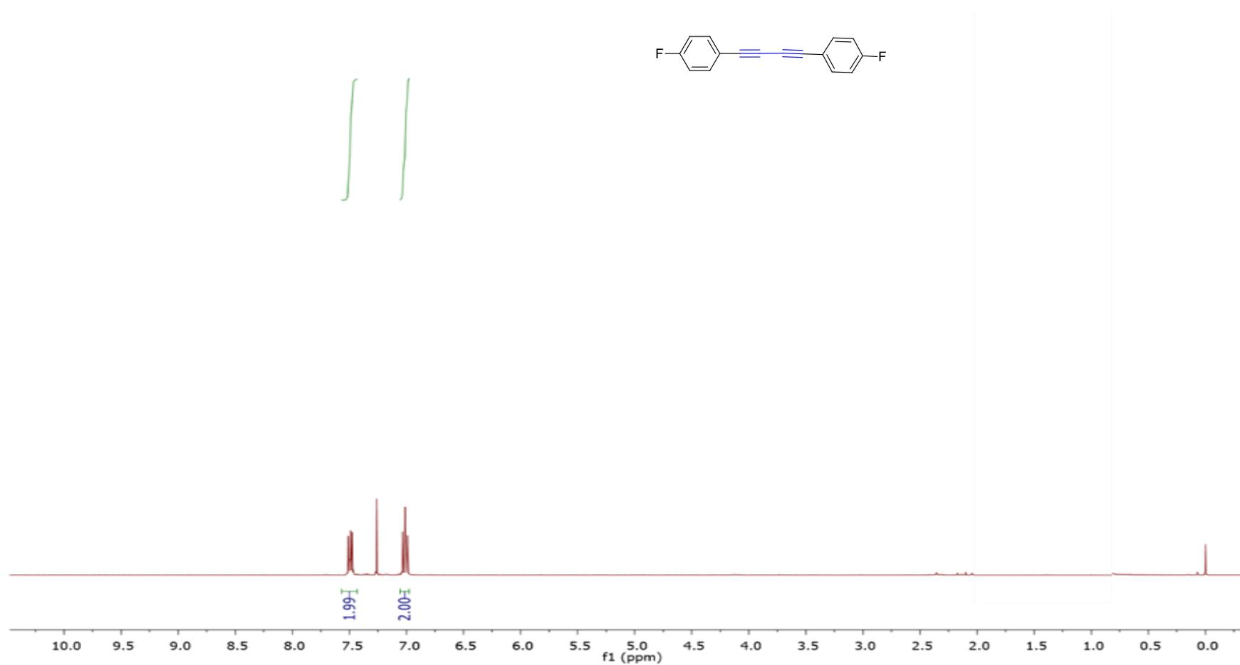
Fig. 17.  $^1\text{H-NMR}$ -spectrum of compound **2i** (500 MHz,  $\text{CDCl}_3$ , 298K)
