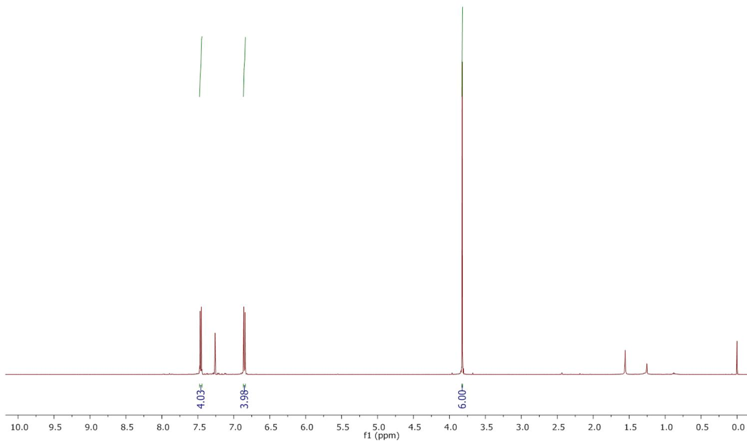
Fig. 5. <sup>1</sup>H-NMR-spectrum of compound **2c**<sup>1</sup>(500 MHz, CDCl<sub>3</sub>, 298K)
