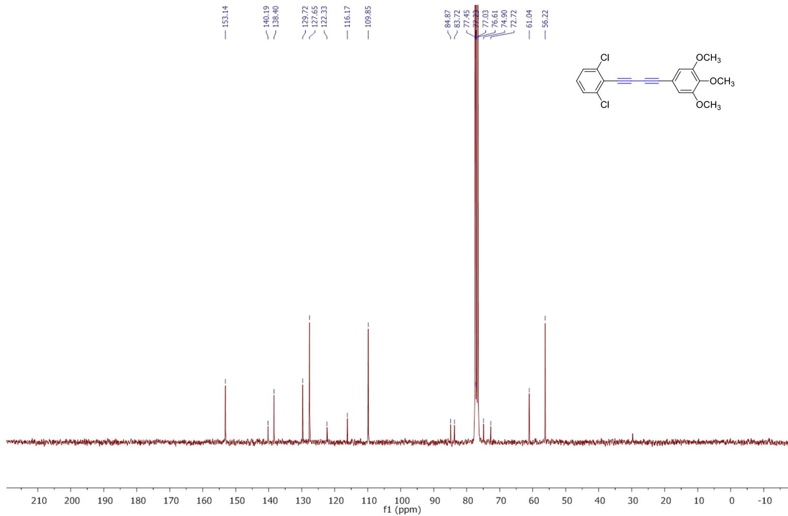
Fig. 36.  $^{13}\text{C}$ -NMR-spectrum of compound **2r** (101 MHz,  $\text{CDCl}_3$ , 298K)
