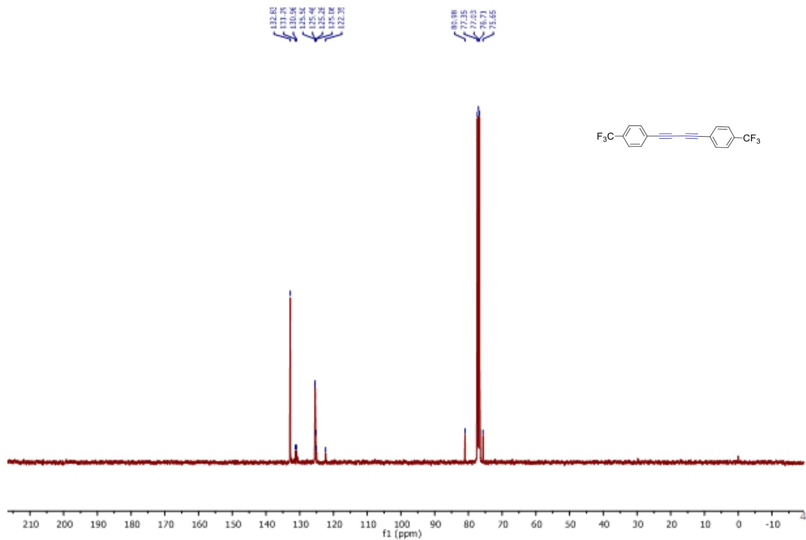
Fig. 22.  $^{13}\text{C}$ -NMR-spectrum of compound **2k** (101 MHz,  $\text{CDCl}_3$ , 298K)
