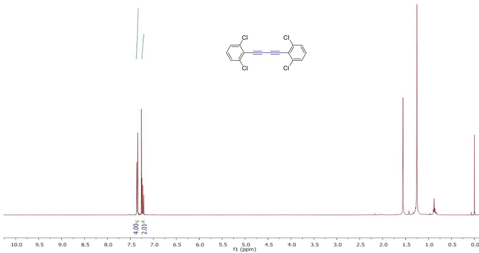
Fig. 23.  $^1\text{H-NMR}$ -spectrum of compound **21** (400 MHz,  $\text{CDCl}_3$ , 298K)
