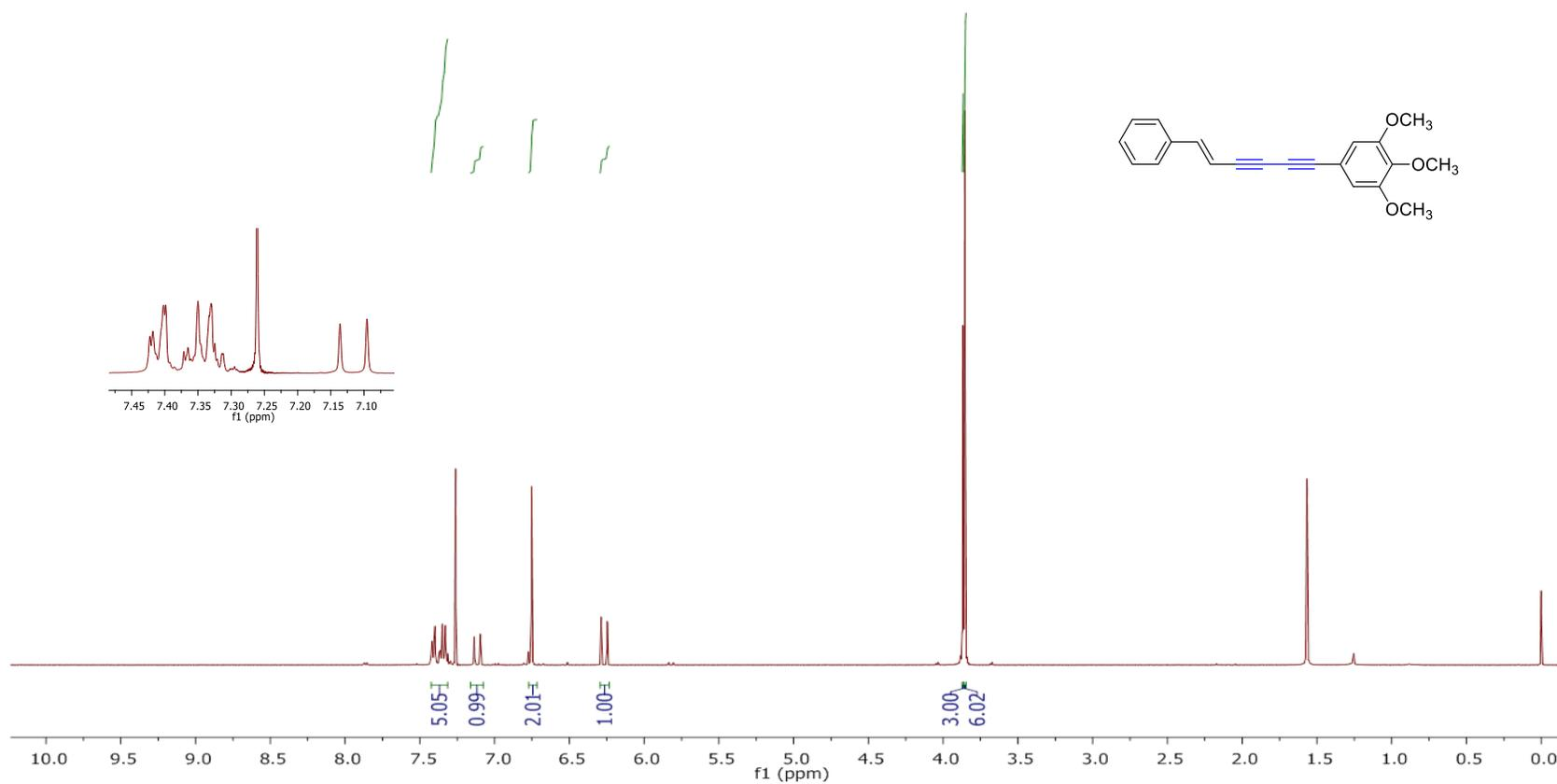
Fig. 37.  $^1\text{H}$ -NMR-spectrum of compound **2s** (500 MHz,  $\text{CDCl}_3$ , 298K)
