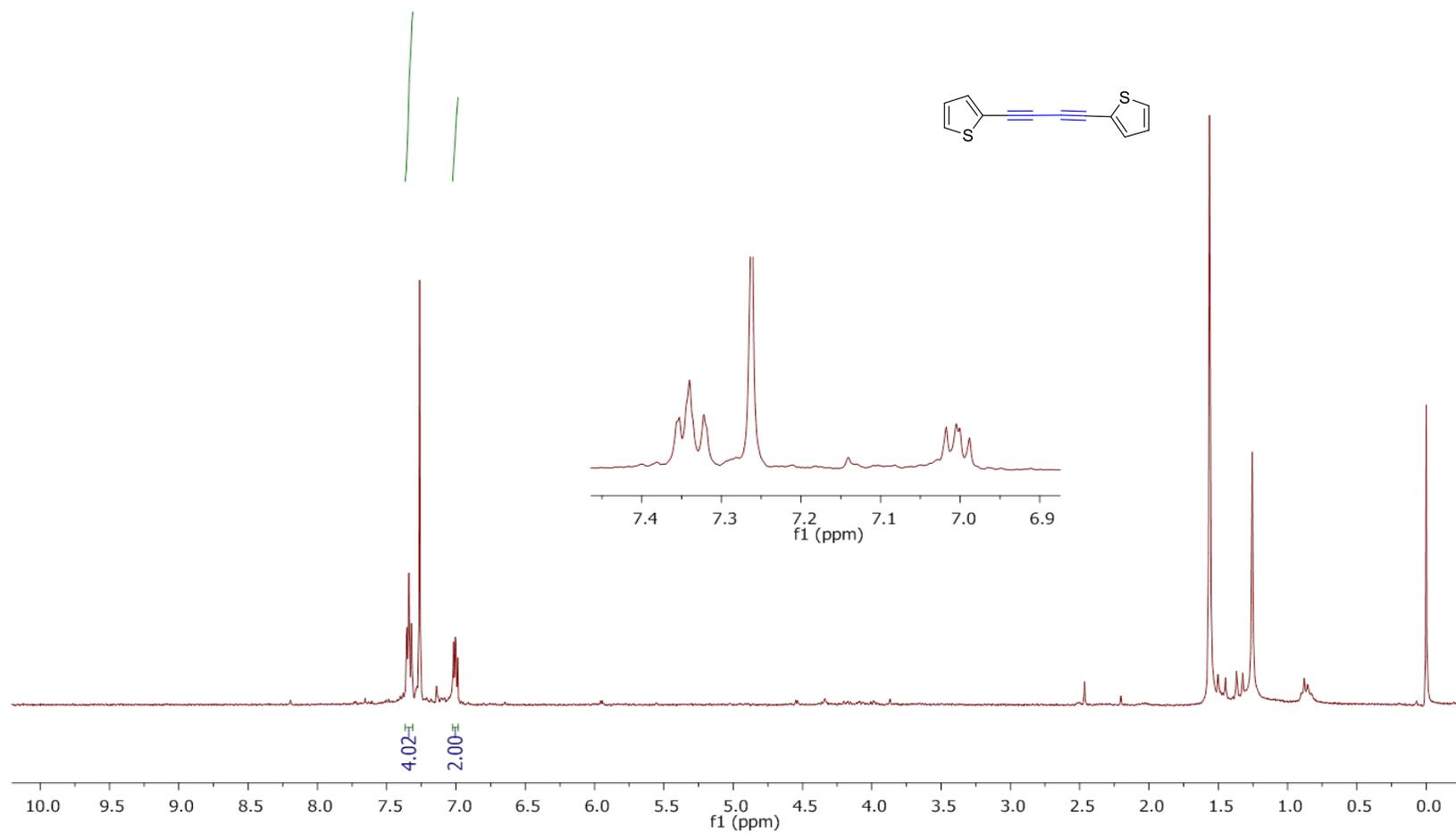
Fig. 29. <sup>1</sup>H-NMR-spectrum of compound **2o**<sup>1</sup> (400 MHz, CDCl<sub>3</sub>, 298K)
