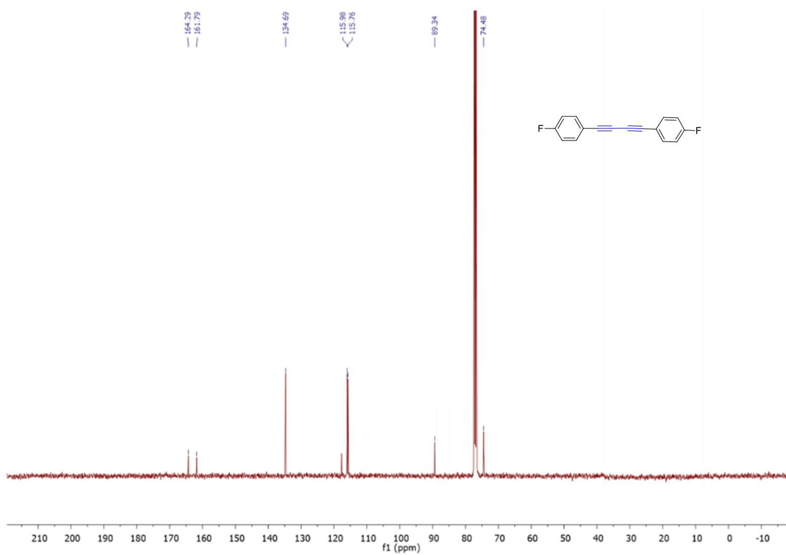
Fig. 18.  $^{13}\text{C}$ -NMR-spectrum of compound **2i** (101 MHz,  $\text{CDCl}_3$ , 298K)
