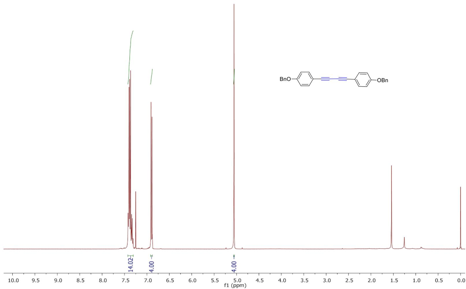
Fig. 11. <sup>1</sup>H-NMR-spectrum of compound **2f<sup>1</sup>** (400 MHz, CDCl<sub>3</sub>, 298K)
