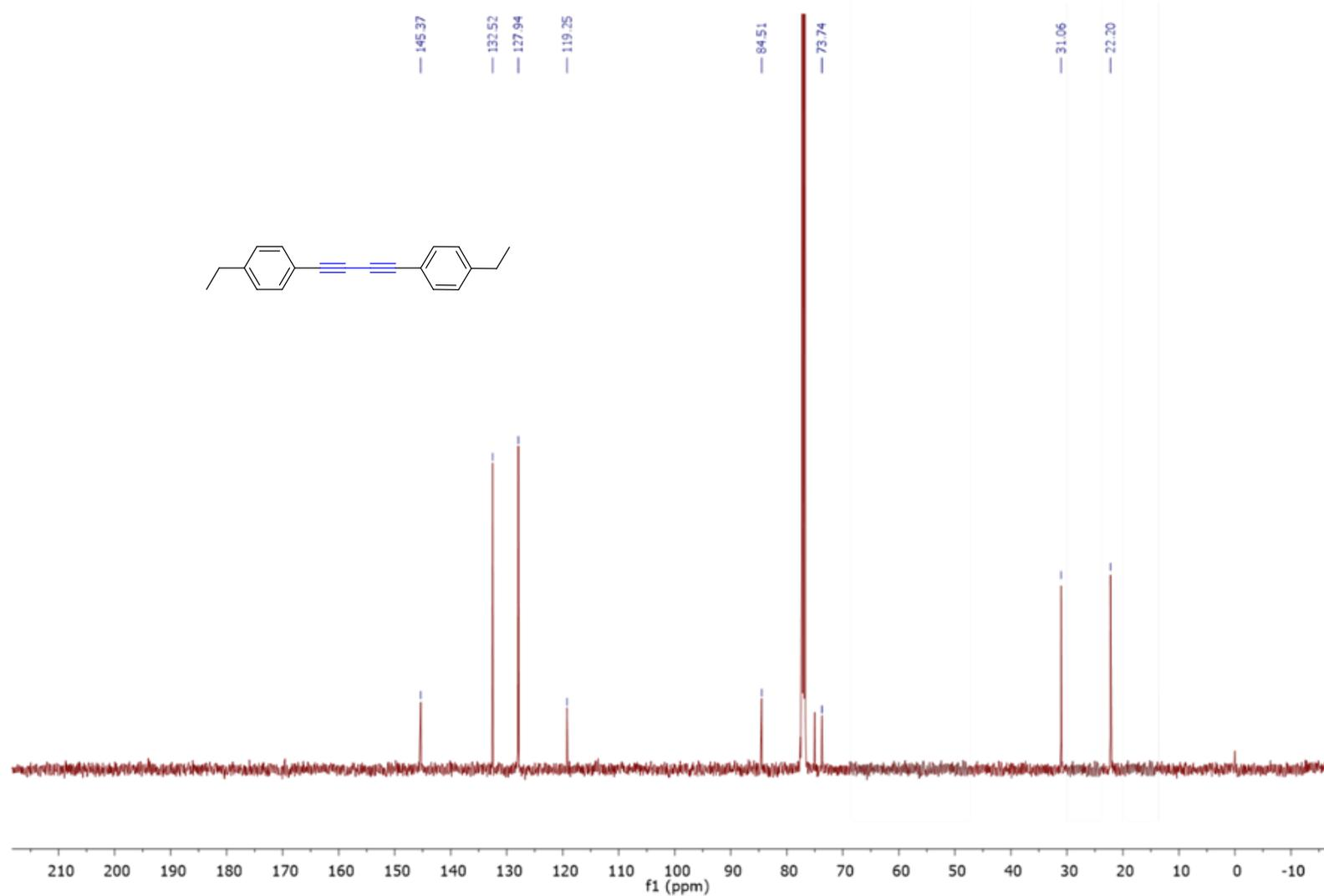
Fig. 10. <sup>13</sup>C-NMR-spectrum of compound **2e** (101 MHz, CDCl<sub>3</sub>, 298K)
