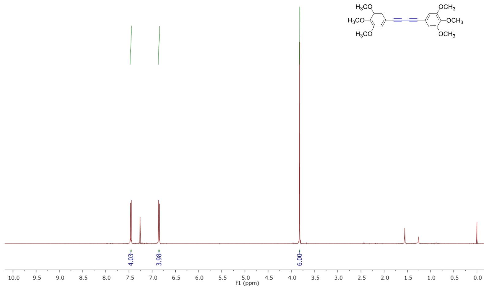
Fig. 1.  $^1\text{H}$ -NMR-spectrum of compound **2a**<sup>1</sup> (400 MHz,  $\text{CDCl}_3$ , 298K)
