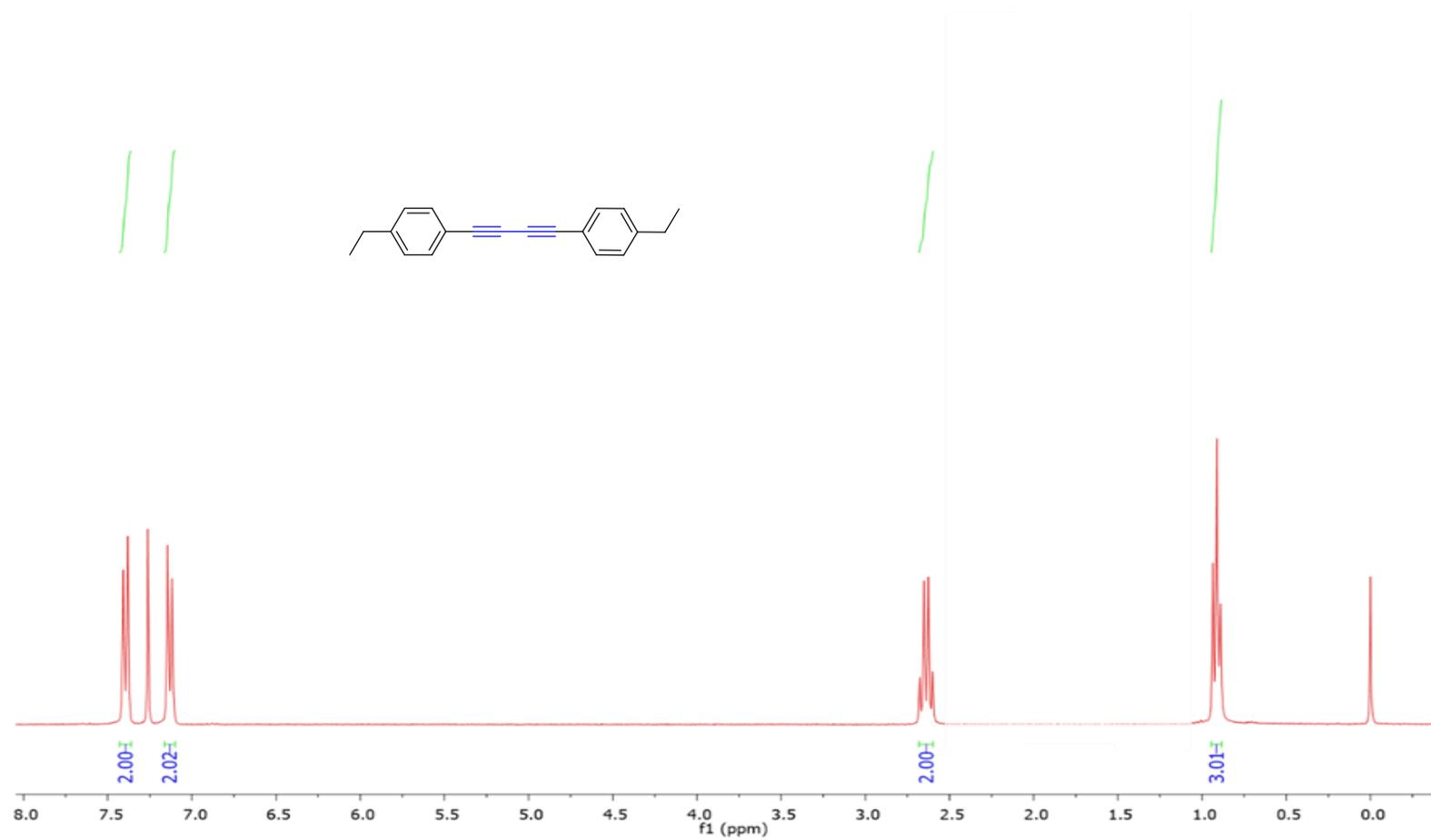
Fig. 9. <sup>1</sup>H-NMR-spectrum of compound **2e** (500 MHz, CDCl<sub>3</sub>, 298K)
