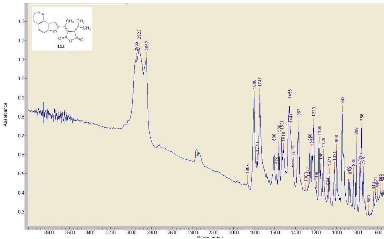
Figure S32: The IR spectra of **12**.
